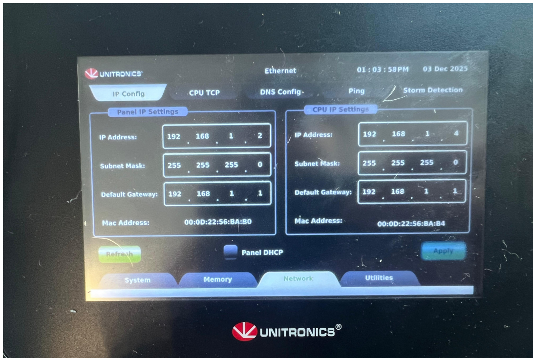
FIGURE 5.34 – Configuration Ethernet de l'automate
