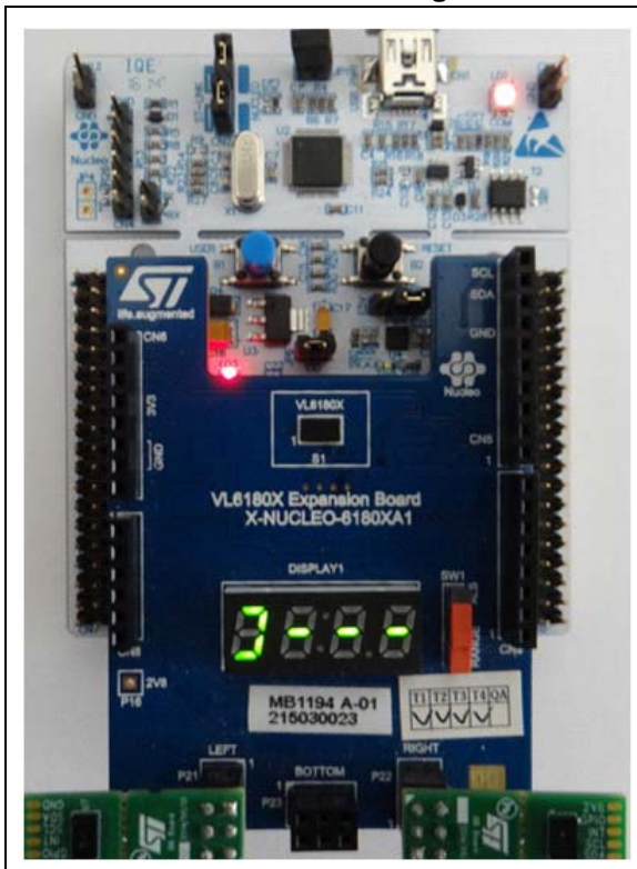
Figure 33. STM32 Nucleo, VL6180X expansion and two VL6180X satellites boards - "GestureDetect1" configuration
