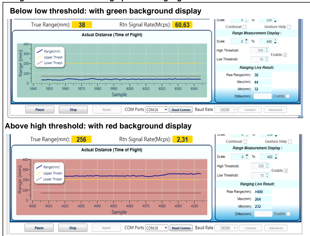
Figure 50. Actual distance graphs showing high and low thresholds
