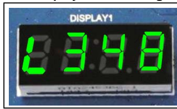
Figure 27. Left digit of the display if ambient light value above 1000 Lux
