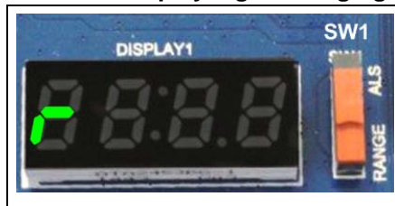
Figure 13. Left display digit in ranging mode
