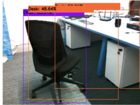
Figure 1. Example object detection by the MobileNet model. In this example, the model captured the chair with reasonable accuracy. However, the bounding box for the desk was not very accurate since it also captured the chair.
