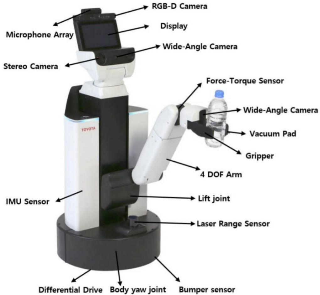
Figure C.1: Sensors and actuators of the Toyota HSR robot [Yi+20b].
