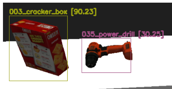
Figure 3.4: Inference on two objects of the dataset, inside the simulator. Caption of the bounding boxes: object_class [accuracy of the prediction].
