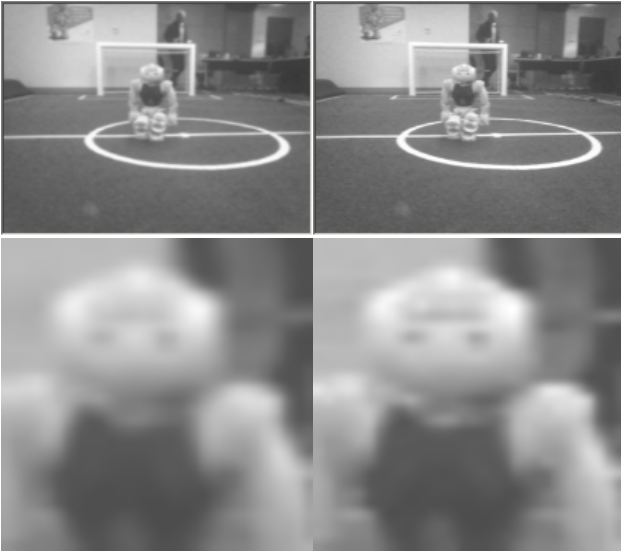
Figure 2: Downsampled images at level 5 of the pyramid using slow (top left) and fast (top right) methods. Bottom row zooms in on the robot to highlight differences between slow (bottom left) and fast downsampling approaches. NAO’s pixelated shoulder is clearly visible, showing gradient information loss in fast method.
