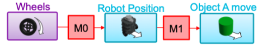
Fig. 6: Illustration of nested models for setup fig.3. To push an object, the robot needs to control its position, and therefore command its wheel.
