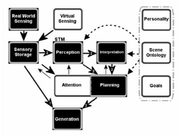
**Fig. 1**. The general framework that embeds the current scenario. Large arrows indicate the direction of information flow, small arrows denote control signals, while arrows with dashed lines denote information availability from modules associated with long term memory. Modules with a white background are not applicable to the scenario described in this paper.
